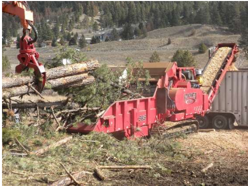
B66 Rotochopper processing wood mulch.
